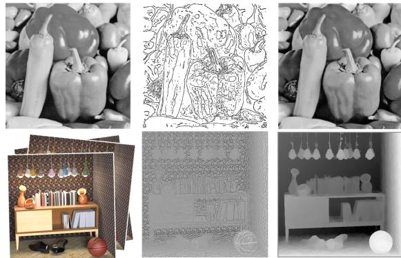
Fig. 1: Top: Elder showed that a representation of image edges including position, brightness and contrast, gradient, and blur scale is complete as it lets us reconstruct the image via a diffusion process with low error. Left to right: Original image, edge locations, reconstructed image; reproduced from [27]. Bottom: We show that a similar approach is possible for multi-view images and provides a complete representation for scene geometry via depth.
