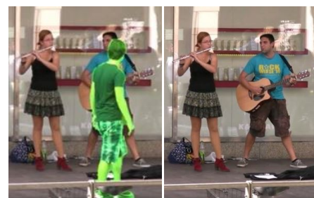
Video inpainting of dynamic objects. An occluding passerby is removed, and the unknown motions of the musicians behind are created by seamlessly recombining other parts of the video.
